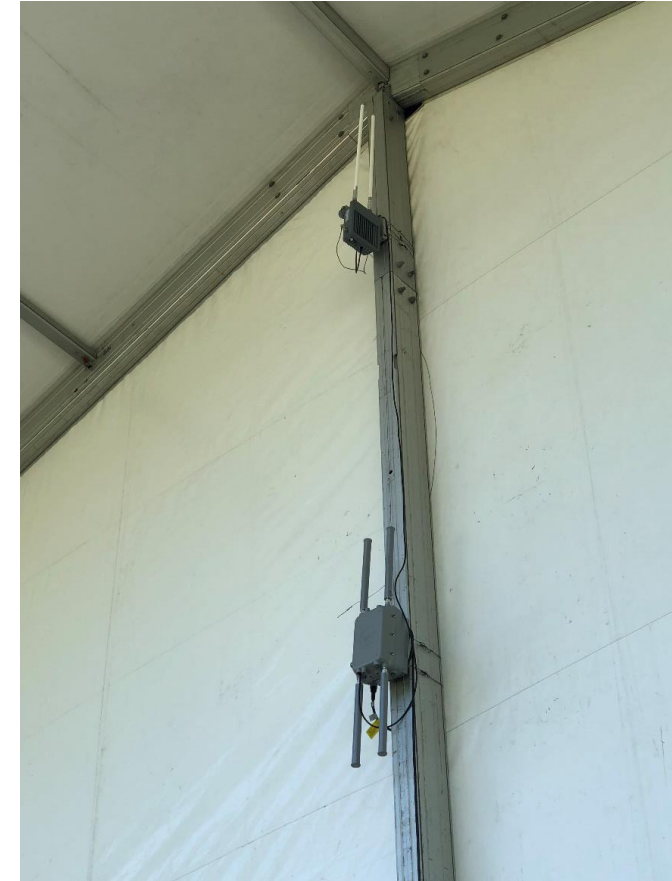
Cisco LoRaWAN gateways placed at the apex of tents used to house the MDM 2018 expo.
